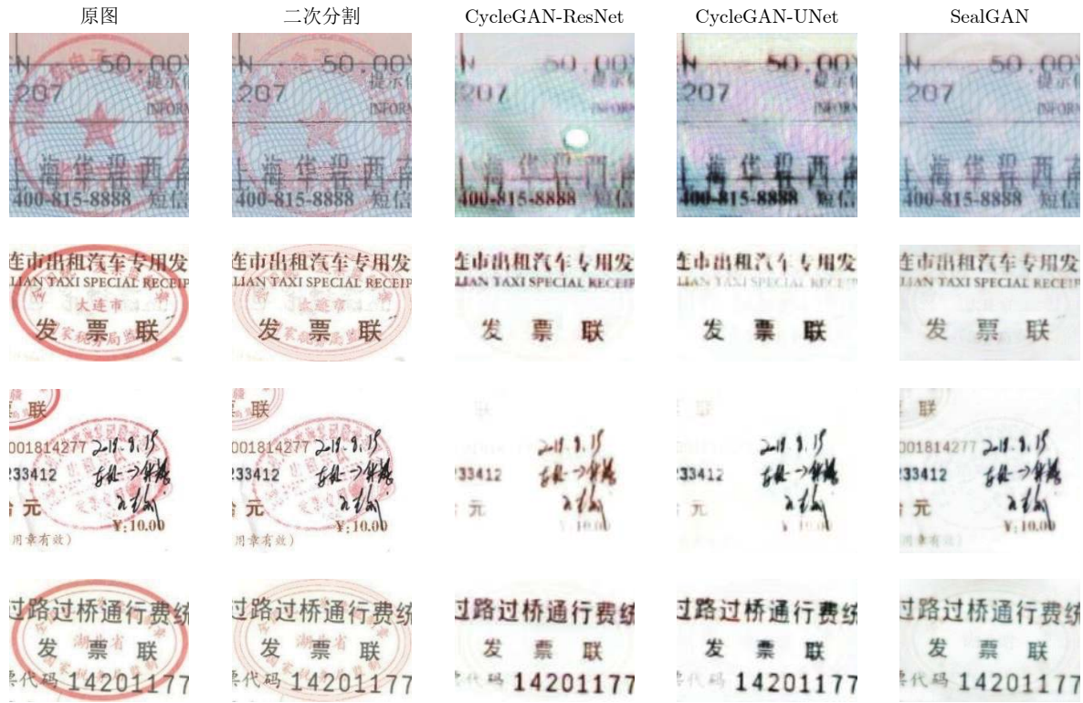
图 8 基于二次分割、CycleGAN-ResNet、CycleGAN-UNet 和 SealGAN 的印章消除对比 Fig.8 Comparsion of effect of the seal elimination based on re-segmentation, CycleGAN-ResNet, CycleGAN-UNet and SealGAN
