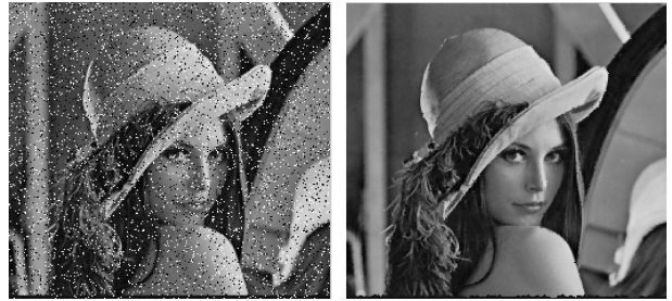
图 2 10% 椒盐噪声污染的 Lena 图像及滤波后结果 Fig. 2 Lena image corrupted by 10% salt & pepper noise and the filtering result
