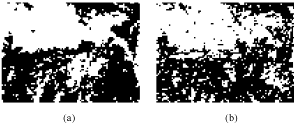
图 10 单波段单极化数据 (唐家山地区 SAR 图像 2) ((a) 基于像素的变化检测图; (b) 似然比算法变化检测图)) Fig. 10 The single band and single-polarization data (the second group of SAR images of Tangjiashan area) ((a) Change detection image of pixel-based method; (b) Change detection image of likelihood ratio method)
